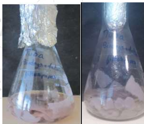
Figure 6: Showing degradation of filter paper
