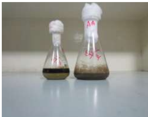
Figure 6: Day by day oil degradation activity on seventh day by culture C2 which degrade oil completely (Mobil oil was used)
