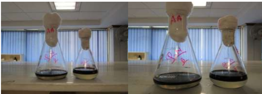
Figure 5: Oil degradation activity on fifth and 7 th day by culture C2 (Mobil oil was used)
